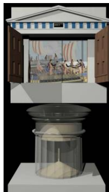
Fig.7: 3D digital reconstruction model of Heron's fixed theatre. Source: (Steadman, 2021, Fig. 3.2).
