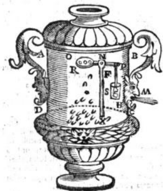
Fig.5: Drawing of Heron's holy water dispenser, vending machine. Source: (Rossi, 2016, fig. 6).
